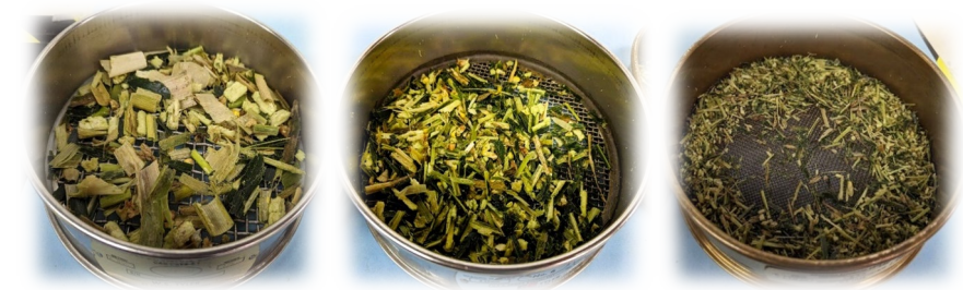
Figure 2. Corn silage particles separated by screen sizes of 1.5875 mm (1/16"), 3.175 mm (1/8"), and 6.35 mm (1/4").
