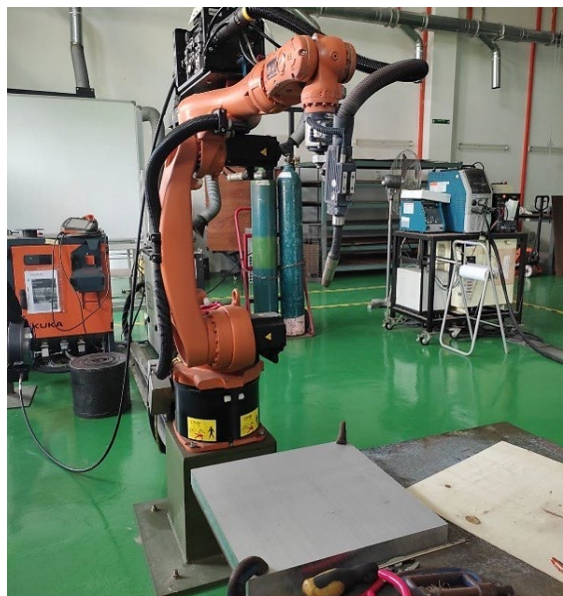
Figure 1. An EWM 352 alpha Q GMAW heat source attached to KUKA KR 5 with EWM M drive 4 Rob 2 wire feeding system.
