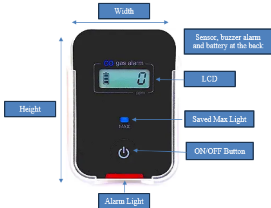
Figure 2. Features of carbon monoxide detector.
