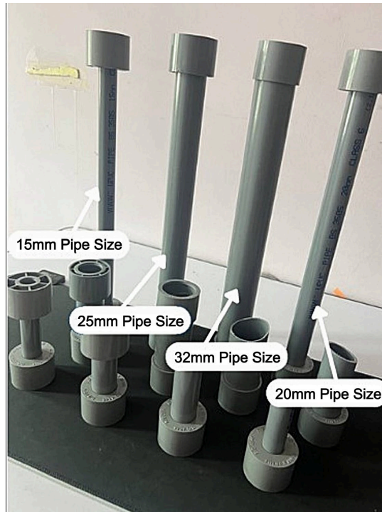
Figure 4. Different sizes of PVC pipes use in the project.
