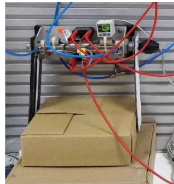
Figure 12. Digital SMC pressure switch display pressure value in green.
