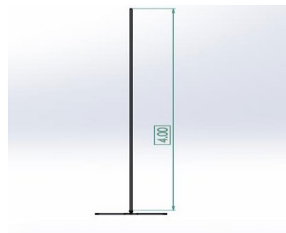
Figure 3. PVC pipe for water head simulation.
