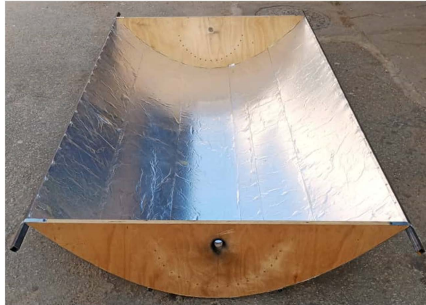
Figure 2. Fabricated solar parabolic trough.
