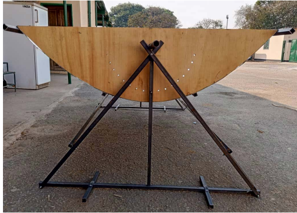
Figure 7. Manual tracking system of the fabricated PTSAH.
