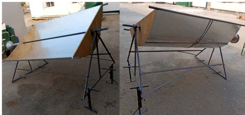
Figure 6. Different views of the PTSAH assembly.
