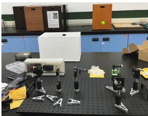
Figure 1. The setup for Michelson Interferometer shows the arrangement of components where the interference pattern (green circle) is observed.
