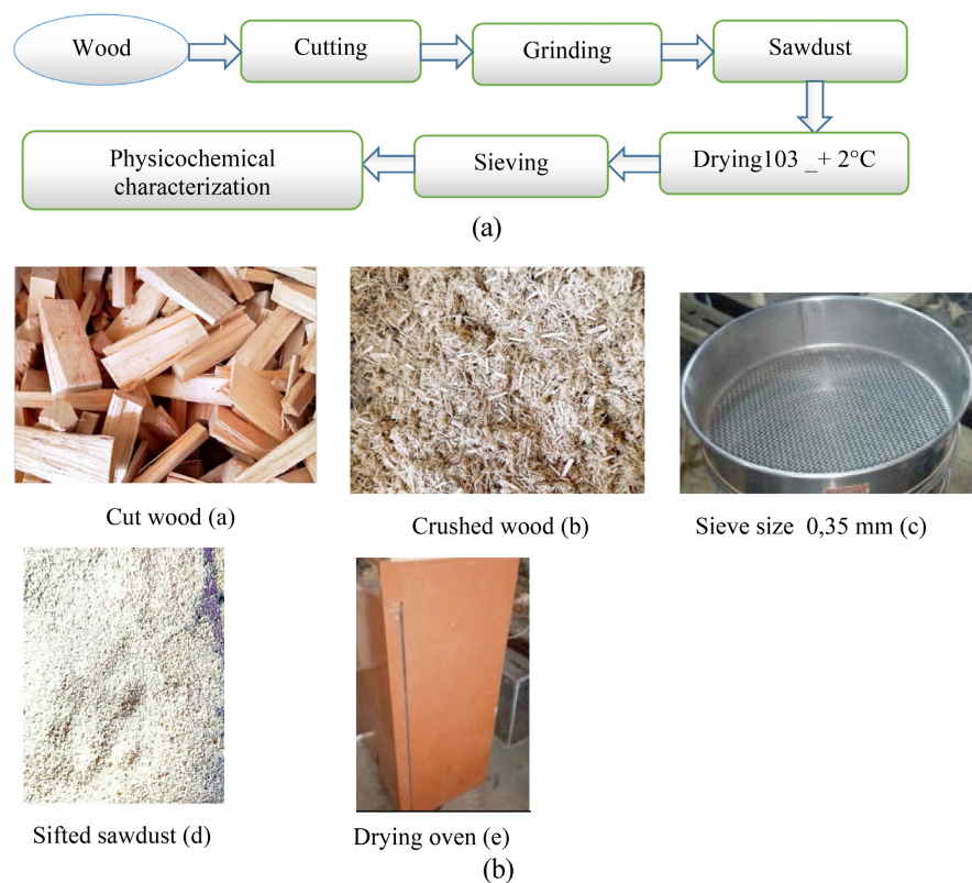
Figure 1. (a) Diagram of the Ayous sawdust preparation process; (b) Preparation of Ayous sawdust.
