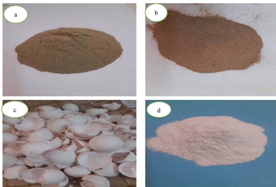
Figure 1. Image of (a) clay 1 (b) clay 2 soil and (c) eggshell waste (d) eggshell powder.
