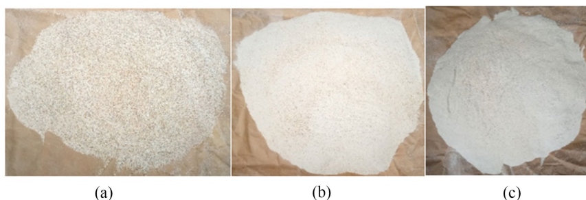
Figure 2. Ground horns separated into different sizes. (a) 300 µm; (b) 100 µm; (c) 50 µm.
