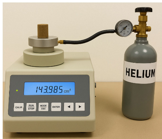
Verification by Gas Pycnometer (Helium Method)
