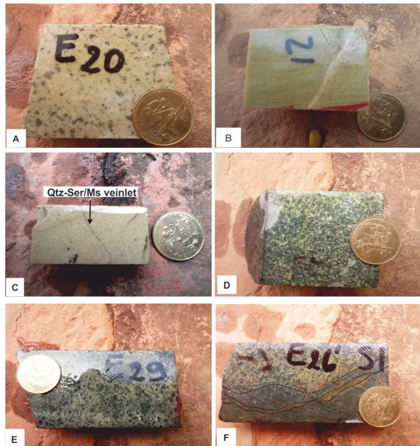
Figure 3. Macroscopic view of altered rocks from Diénéméra-Gongondy copper deposits. Sericitic alteration 1 affecting microdiorite porphyry at Gongondy (A). Sericite alteration 2 affecting dacitic rocks: Pervasive alteration (B) and alteration saw in veinlet (C). Propylitic alteration affecting Quartz porphyry microdiorite in Diénéméra (D). Phyllito-carbonate alteration affecting microdiorite in Gongondy deposit (E). Chloritic alteration affecting porphyry microdiorite in Gongondy (F).
