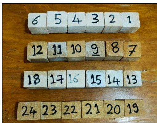
Figure 5. The sandstone samples after consolidation.
