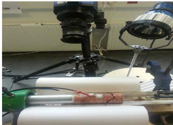
Figure 3. Experimental device of the dynamic tensile test by palling.
