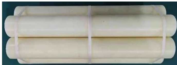
Figure 16. Bundled solid propellant plastic rods of the same specifications.
