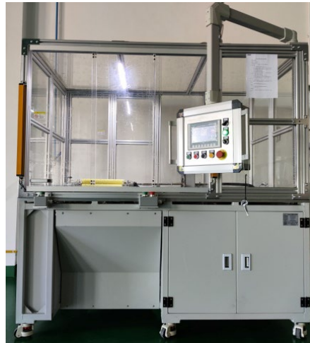
Figure 15. Physical equipment for automated strapping of solid propellant.
