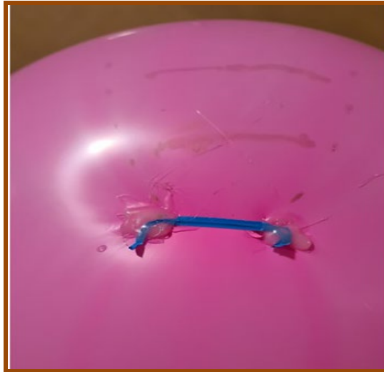
Figure 1. Illustration of how a constraint affects the curvature of an expanding surface. The wire attached at two points limits expansion, causing an inward curvature of the balloon surface (reproduced from [14]).
