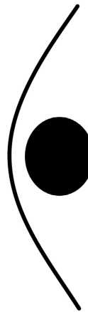
Figure 7. The sweeping shock wave edges (approximated) and the bow wave of the entire body are shown.
