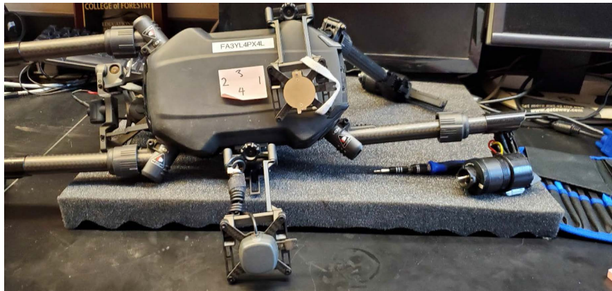
Figure 3. Matric 200 platform during laboratory damage inspection.
