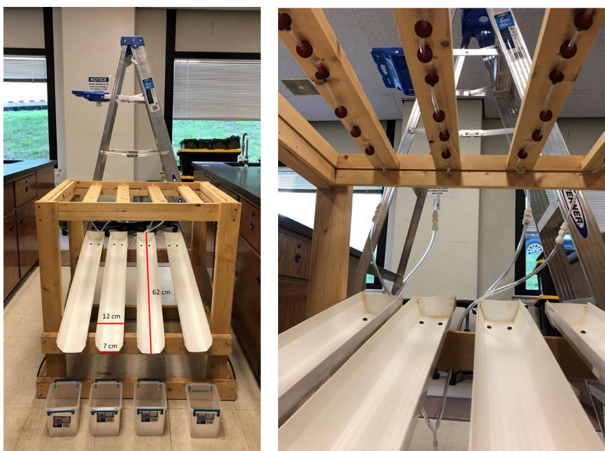
Figure 1. Images of the rainfall-runoff simulator (left) with additional angle to view the drip-emitters and tubing (right). The white trays were set at a slope of 22.1%. Tea bags containing the soil-fertilizer treatment combinations were placed on the white trays directly below the four down-slope drip emitters. Images adapted from 2021 photographs by M. Morrison.
