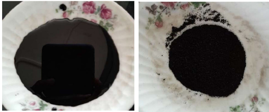
(a) Oily sludge before pyrolysis at 400°C for 30 min
