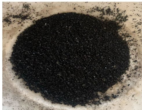
Figure 6. Coal obtained after pyrolysis of the sludge at 400°C for 1 hour.
