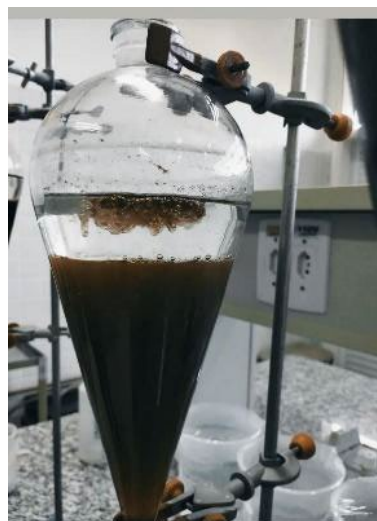
Figure 3. Lipid material from landfill leachate retention in hexane top layer in liquid-liquid extraction.
