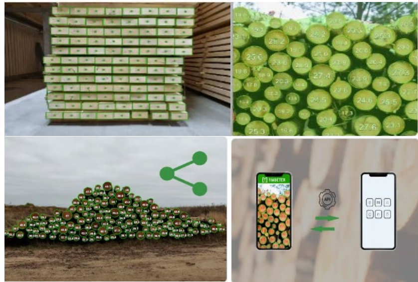
Figure 1. Measurement with Artificial Intelligence (AI) by the company Timbeter.
