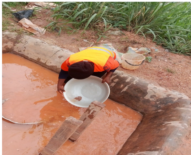
Figure 13. Gold processing in cemented sink.
