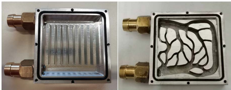
Figure 20. CNC processed 2 mm microchannel and TO channel LCPs.
