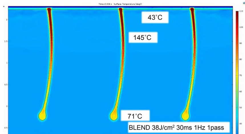
Figure 6. Simulation of hair heating for skin type IV and dark thick hair in maximum operating conditions with a triple wavelength (Blend) laser of 810 + 940 + 1060 nm.
