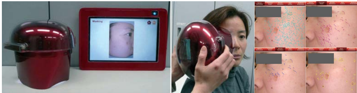
Figure 3. Magic Ring facial imaging system and image analysis overlays of facial skin texture, pores, wrinkles, skin tone, and hyperpigmented spots.
