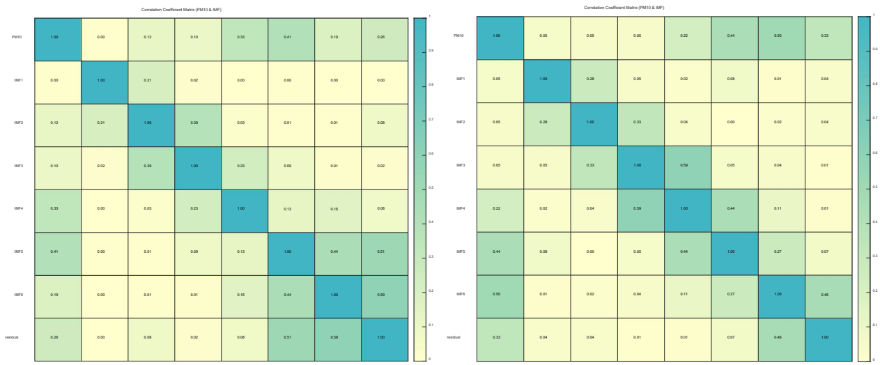
Figure 5. Correlation between EEMD-decomposed GNSS ZNHD IMF components and PM 10 concentration. Left: BJFS station; Right: CHAN station.
