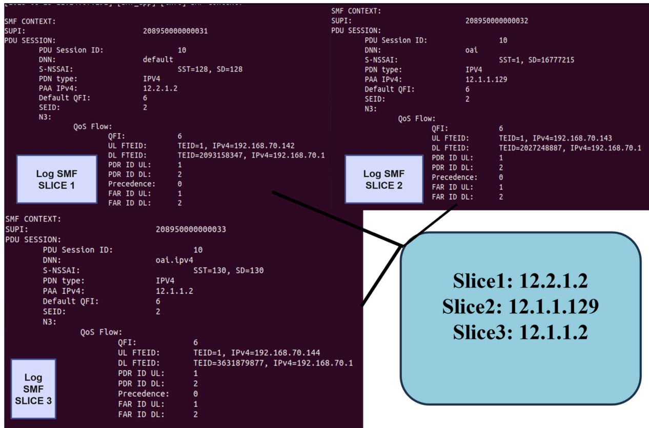
Figure 6. Image illustrating the establishment of the PDU session for each of the 3 slices.
