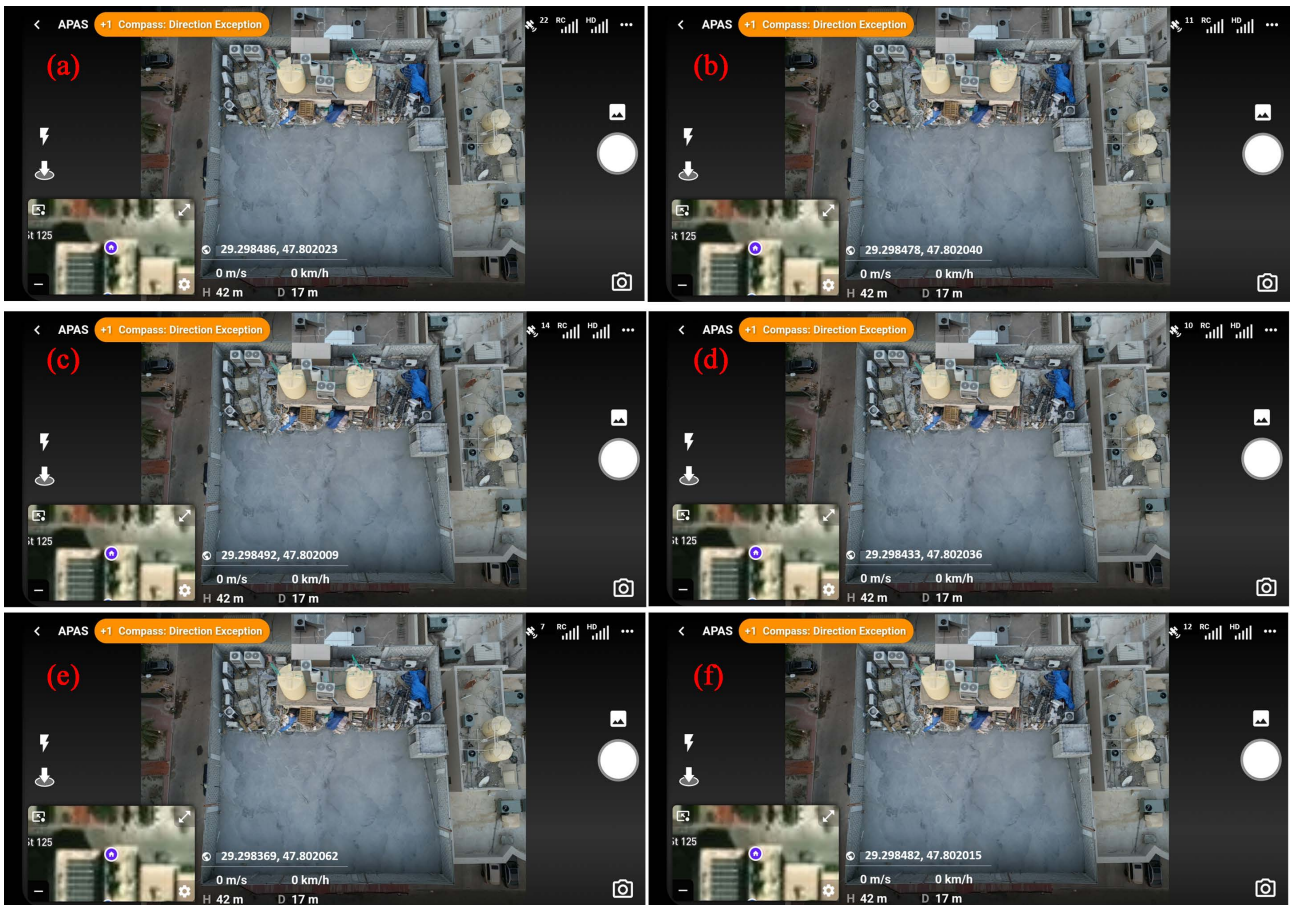
Figure A1. Capturing Location Building using Drones for Single Satellites System. (a) All Enabled, (b) GPS-Only, (c) Gloanass-Only, (d) Galiloe-Only, (e) SBAS-Only, (f) BeiDou-Only.
