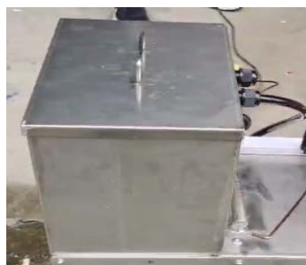
Figure 11. Corrosion-resistant liquid tank.
