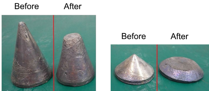
Figure 3. The physical diagram of the loss of the lead cone.
