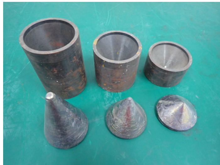
Figure 5. The physical picture of the molds and the cast lead cones.
