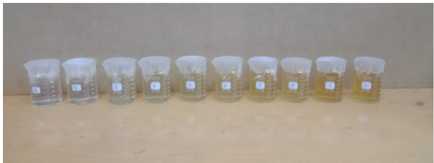
Figure 1. Liquid water-gelatin mixtures at different concentrations of dry gelatin, from lower to higher from left to right.
