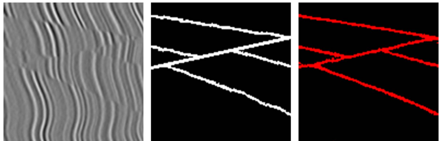
Figure 5. Seismic profile, mask and SAM segmentation results.
