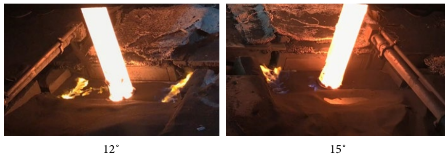
Figure 16. The fluctuation cloud diagrams of liquid steel on the free surfaces of slab mold under different immersion nozzle inclination angles.
