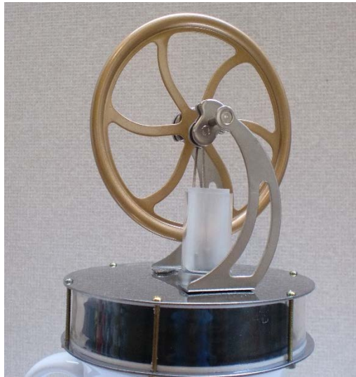
Figure 2. A low temperature Stirling engine (LTSE) works with heat flows (entropy flows) in NISs.
