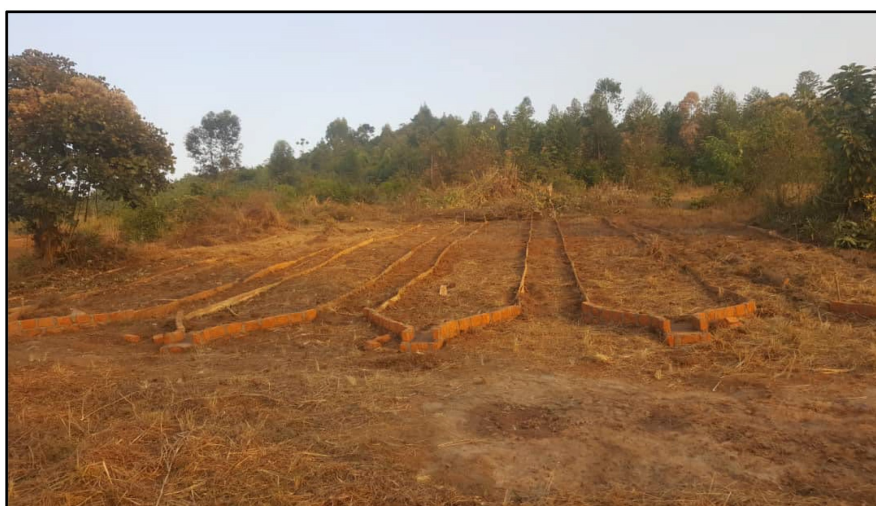
Figure 2. Runoff plots established on farmers' gardens in the Katonga Micro-catchment.
