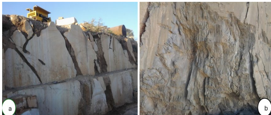
Figure 4. Marble quarry wastes, due to cavities and the presence of shist respectively.
