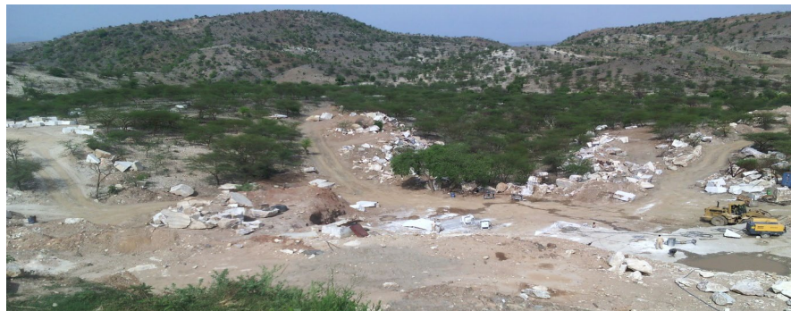
Figure 8. Wastes can be generated due to overburden removal.
