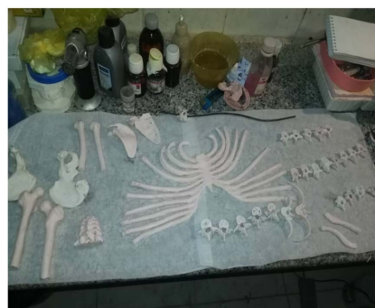
Figure 4. The fabricated skeletal parts made with bone equivalent materials before the construction.
