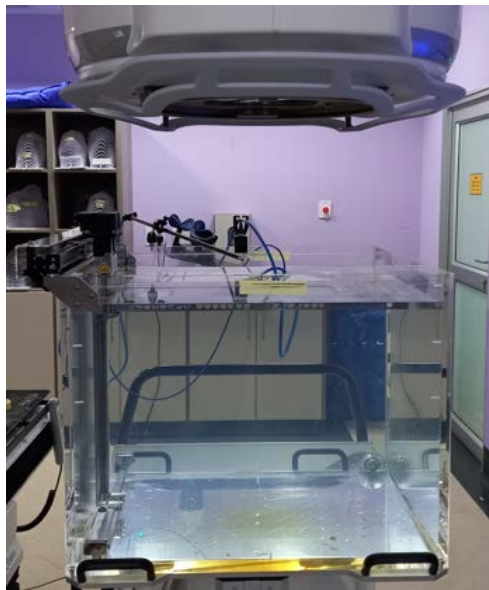
Figure 3. PTW 3D water tank employed for measuring beam profiles and field output factors.
