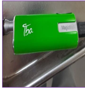
Figure 5. MagicMaX analog-to-digital converter.
