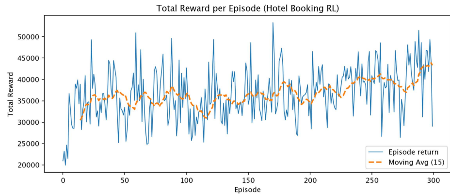
Figure 12. Total reward per episode in the hotel_booking environment. Raw episode returns are noisy, but the moving average (orange line) shows a clear upward convergence.
