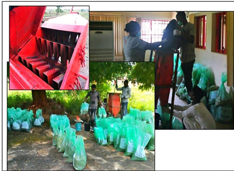
Figure 6. Ripple splitter, splitting and tagging of suspected phosphate horizons.
