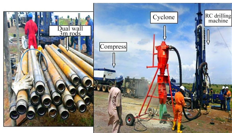
Figure 2. Multipurpose Comacchio Geo 602 Explorer complete with riffle splitter.
