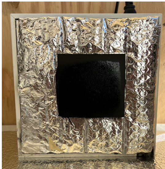
Figure S1. The Keenwise Heater with the outer portion covered with aluminum foil insulation. The inner 4-inch by 4-inch center painted black was used to produce the infrared radiation at various temperatures.
