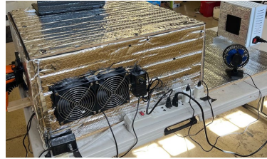
Figure S2. The view from the right side showing the fans and controller for the Seedfactor blanket heater.
