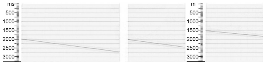
Figure 8. Synthetic time section ( T_0 = 2000 ms, t = 0.2 ms/m) and poststack time, and depth migrations using average velocity V = 1.5 m/ms.
