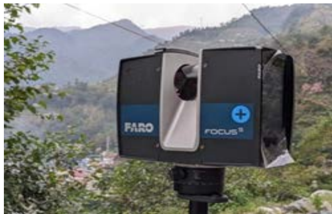
Figure 1. FARO S359+ (Scanner).
