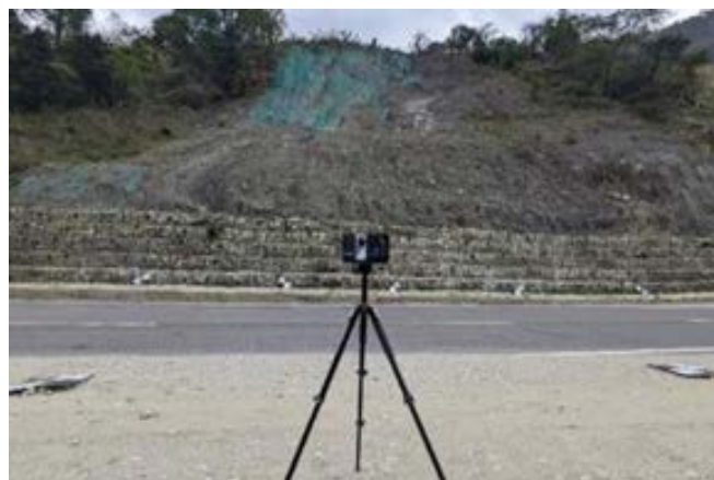
Figure 2. Scanning by FARO S350+ of Kshetrapal landslide.
