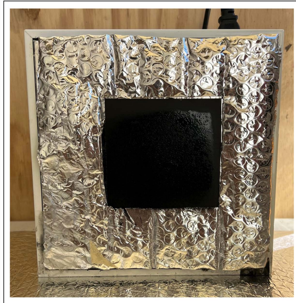
Figure A2. Front view heater facing the test apparatus.
