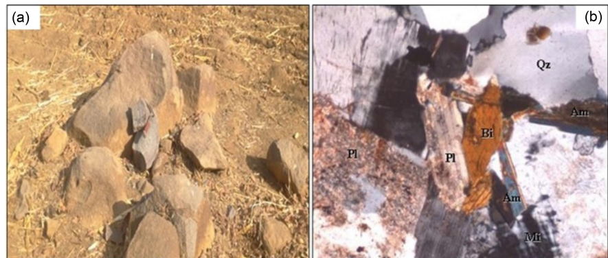
Figure 4. Dougoulogo quartz monzonite. (a) Macroscopic aspects of the Dougoulogo quartz monzonite; (b) Microphotograph of the Dougoulogo quartz monzonite. Qz: quartz; Bi: Biotite; Pl: Plagioclase; Mi: Microcline; Am: Amphibole.
