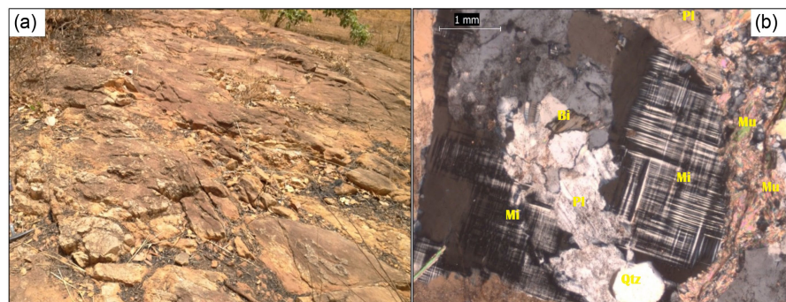
Figure 3. The Ferké two-mica granite in the Banfora belt: (a) Macroscopic appearance of the Ferké granite at the outcrop, (b) Microphotography of the Ferké granite. Bi: Biotite; Mi: Microcline; Mu: Muscovite; Pl: Plagioclase.
