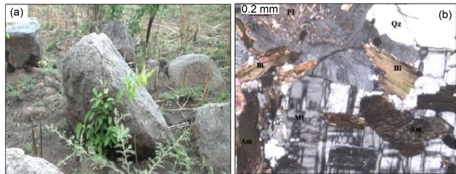
Figure 5. Folonzo granite (a) outcrop of Folonzo granite, in scattered blocks; (b) Microphotograph of Folonzo granite showing essential minerals. Qz: Quartz; Bi: Biotite; Pl: Plagioclase; Mi: Microcline; Mu: Muscovite; Am: Amphibole.
