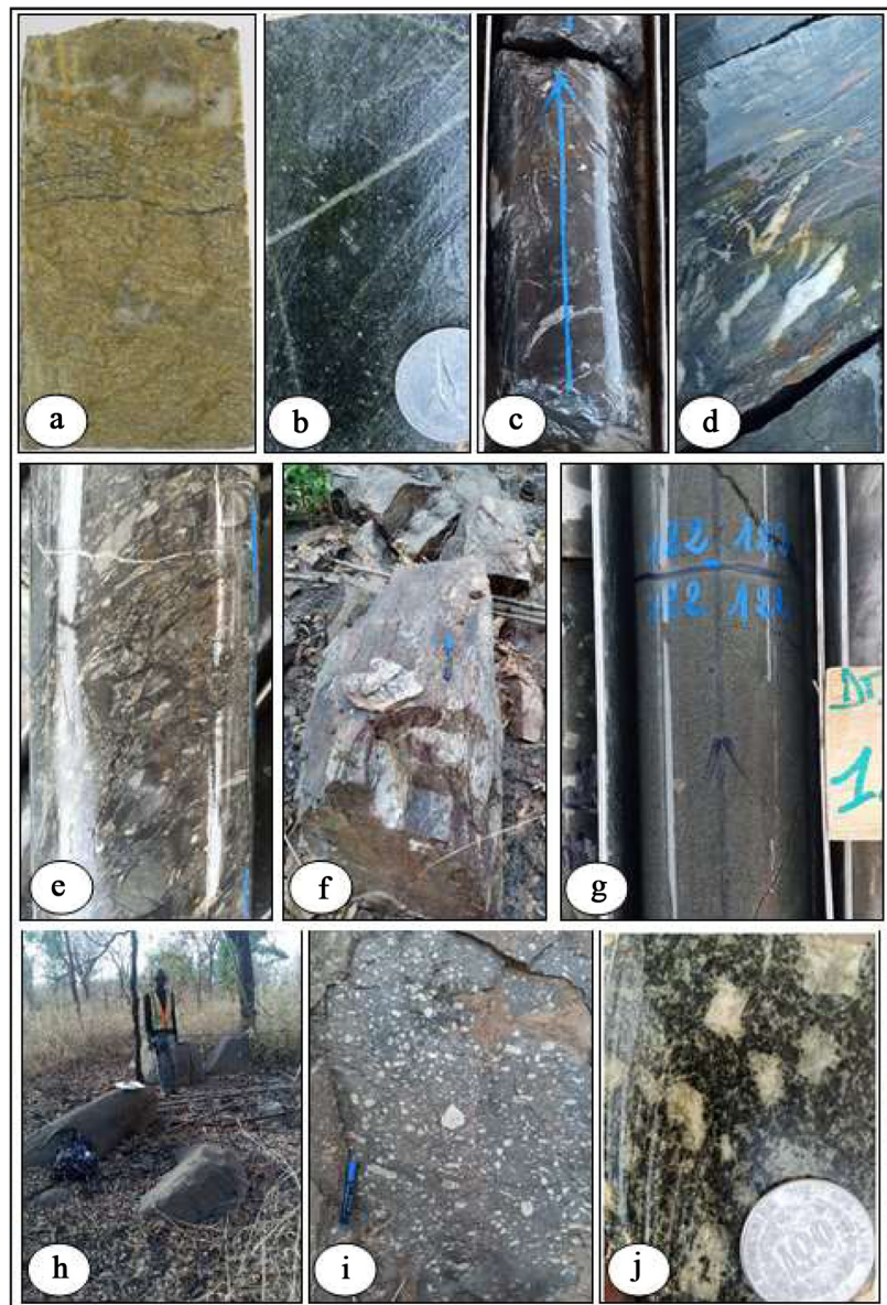
Figure 3. Main lithological units in the Douta permit. ((a), (b)) core of greywackes; ((c), (d)) core of graphitic shales; (e) core of sedimentary breccias; (f) outcrop of cherts benches; (g) core of dolerite; ((h), (i) and (j)) outcrop and core of pegmatitic gabbros.
