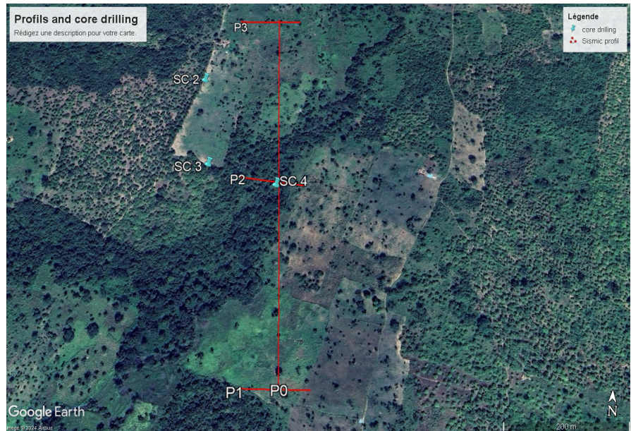
Figure 2. Location of the 4 seismic refraction profiles in the project area. P0 is the baseline.
