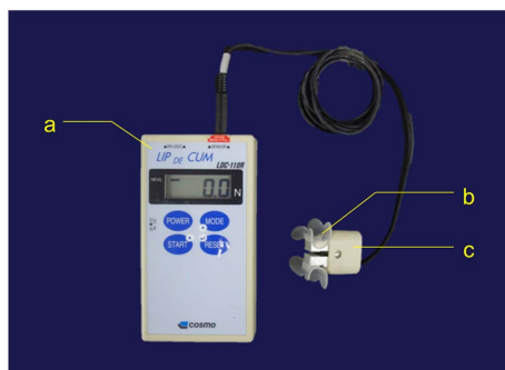
Figure 4. Labial closure strength measurement device (Lip De Cum®). (a) Digital labial closure strength measurement device; (b) Sensor; (c) Holding part (Duckling®).
